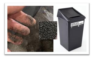
GCS is also in the process of creating an exciting new bio-composite material that combines human hair waste with reprocessed polypropylene to manufacture products for their clients. To date, GCS has produced 5,000 bio-composite hair bins, each containing 1.5 pounds of human hair. The next iteration of their bins will be made using recycled HDPE material sourced from their salons.
